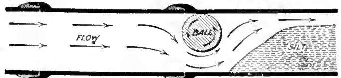
Clogged sewers easily cleaned by flushing through zinc balls.
